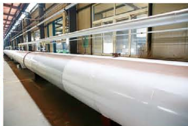
61 米超长硫化罐 61 meter overlength vulcanizer
